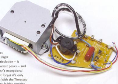
Timestep PSU mod uses a new National Semiconductor LM317L low noise regulator, expensive Vishay rectifiers and premium Nuvotem 'Audio Grade' toroidal transformer...
