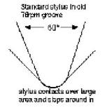
However older 78s were cut to be used with steel needles, on the assumption that the needle would wear down to fit the groove in the first few seconds: when this wider groove is tracked with a 2.5 thou stylus the result is 'bottoming' as can be seen here.
