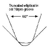
Professional mastering engineers and serious collectors often have a collection of styli sizes, conical truncated as well as elliptical truncated. A good starting point could be:
