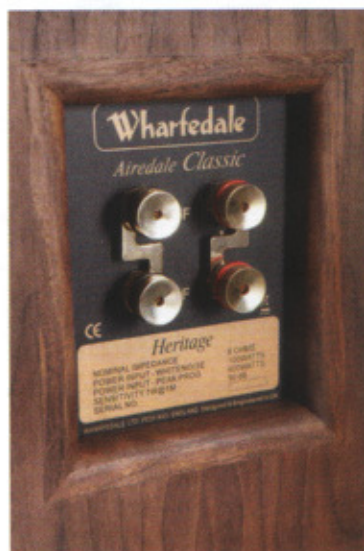
Rear terminal panel carries heavy duty bi-wire terminals with shorting links. They accept 4mm banana plugs, spades and bare wire.
