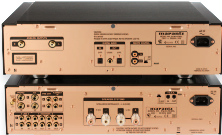
ABOVE: Single-ended analogue and digital outputs on the SACD player (top) join phono, three line and two tape inputs on the amp. Pre-out/power-in are included
